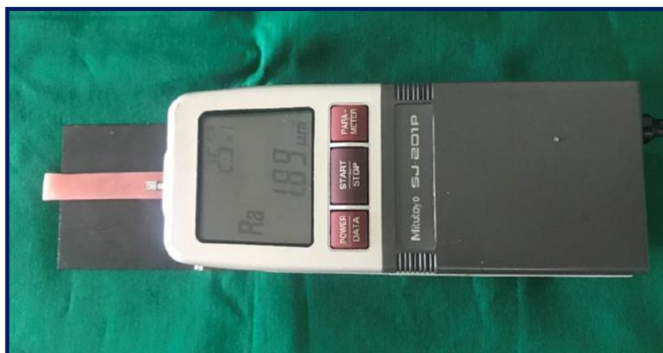
Figure 1. Evaluation of surface roughness using surface Profilometer.
