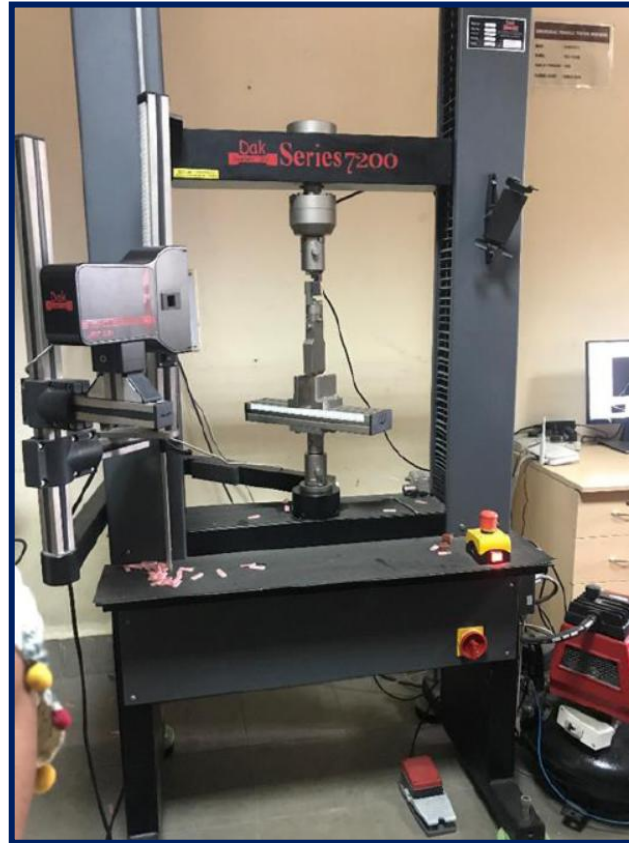
Figure 2. Universal testing machine.
